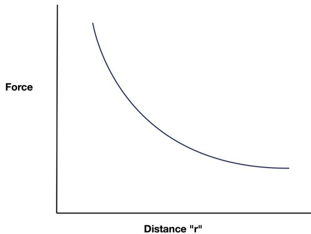
We have already determined that energy is the area under the Force - Distance curve (See the Work - Energy Bulletin.)
